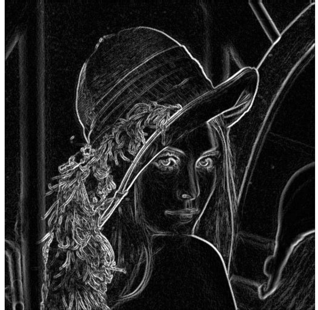
Derivative of Gaussian filtering
