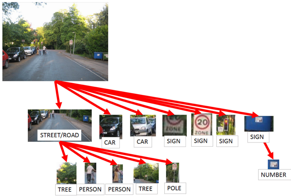
(a) TDVT image representation for a test image. The main objects in the image in descending order of importance are: road, car 1, car 2, and different signs. The road has associated a pair of trees, a pole, and the two persons at the end of the road.
