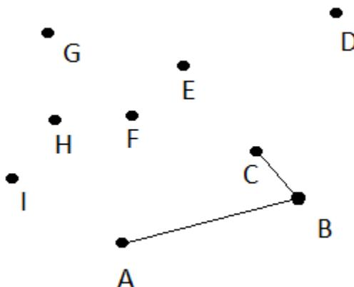
Now, when we consider point D, we see that BCD is a right turn, not a left turn. So, we pop off C from the stack and then look at the turn ABD, since AB are the top two items in the stack. This is a left turn, so our hull changes to ABD. Fast forward and we get to when F gets added to the hull and our picture looks like:
