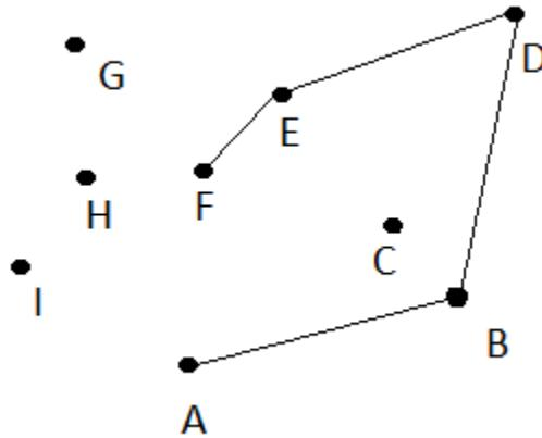
Now, let's consider G. The turn EFG is a right hand turn, so we pop F off the stack. The turn DEG is ALSO a right hand turn, so we pop E off the stack. Finally, we find that the turn BDG is a left hand turn, so our hull is as follows:
