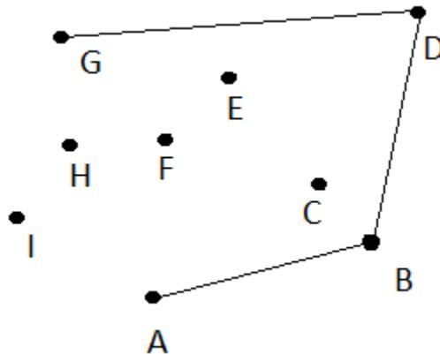
In the second to last iteration, H will get added onto the stack. In the last iteration, H gets popped off the stack and then I gets pushed onto it. Then, the hull is completed by adding the edge IA:
