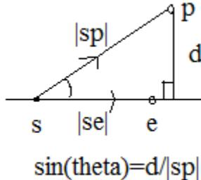
The desired distance is the line drawn from  $p$  down to  $se$  that is perpendicular to  $se$ . This line segment is also the height of a right triangle with points  $s$  and  $p$ . Label the desired distance  $d$ , then  $\sin\theta = \frac{d}{|sp|}$ , so the desired distance is  $d = |sp|\sin\theta$ .
