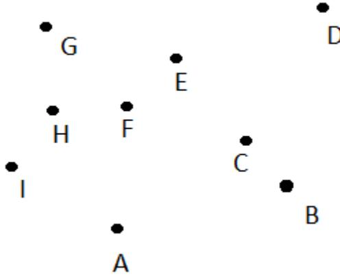
The points are already sorted in alphabetical order based on the criteria given. Point A is the starting point. Initially, the stack contains A, B and C and our hull looks like:
