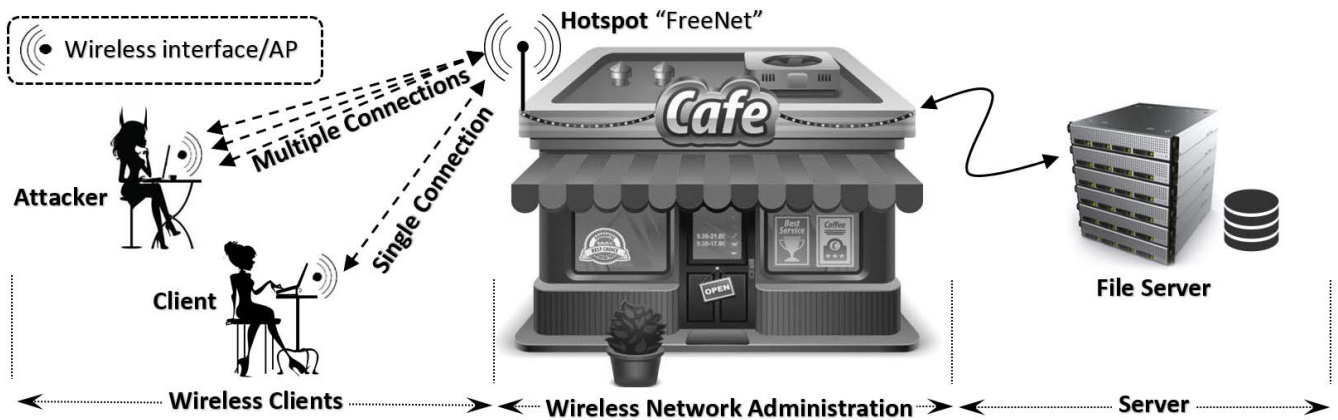
Fig. 2: Proposed attack testbed set up. The attacker and the client used Laptops with TPE-NUSBDB wireless network interface card to connect to the wireless network. Dlink DIR-890L was used as a hotspot and bandwidth controller. We used a Linux based workstation to create the File Server.
