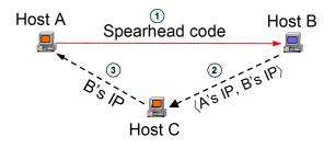
Figure 6.7: The procedure in counterattacking dual-honeypot defense by an advanced twostage reconnaissance worm (host A is the bot under inspection; host C is in A's peer list that has the main-force code.)
