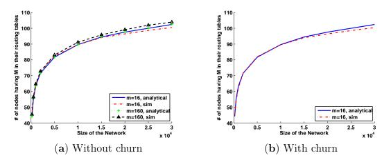
Figure 5.8: Comparison between analytical and simulation results of  $\overline{N}_{routing}$ . The simulated P2P botnet is Kademlia-based with a D(1, 1, 8) routing table structure.
