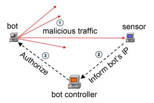
Figure 6.1: Illustration of the procedure of detecting honeypot bots in a centralized botnet
