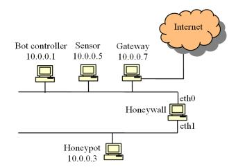
Figure 6.2: Network deployment for honeypot detection experiments
