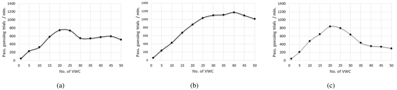
Fig. 5: Comparison between three different APs against our proposed attack where (a) Dlink-DIR890L, (b) ASUS-RT-AC68U (c) Linksys WRT54. The traditional active dictionary attack intensity is represented in the first data point.
