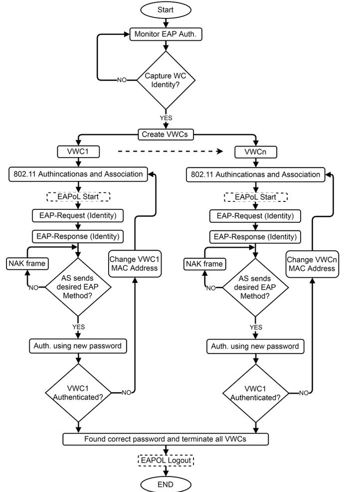
Fig. 4: Our proposed parallel active dictionary attack using one wireless interface card (WIC)
