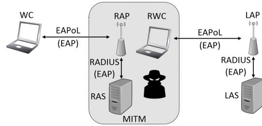
Fig. 1: Typical MITM attack on WPA-II enterprise
