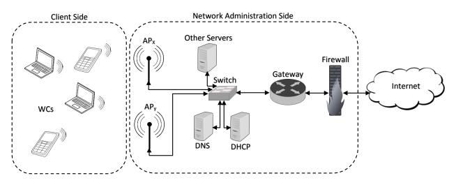
Figure 1.1: Typical WLAN diagram were Wireless clients (WCs) connect to the Internet through Access Points (APs). DHCP and DNS servers are used to assign network configuration and resolve domain names, respectively. The network administrator may add other servers to the network based on the WLAN design, for example, Remote Authentication Dial-In User Service (RADIUS) server. Gateway is used to route network traffic to the Internet while firewall is used to protect the WLAN from the Internet.
