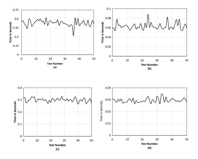
Figure 3.5: ETA detection procedure time duration when  $AP_x$  and  $AP_y$  use the same gateway. (a) connecting to  $AP_x$ . (b) secure 3-way TCP handshake. (c) switching to  $AP_y$ . (d) receiving a response from the web server.
