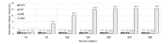
Figure 6.4: Comparison between download data rate for each software (Table 6.1) used in our testbed evaluation.
