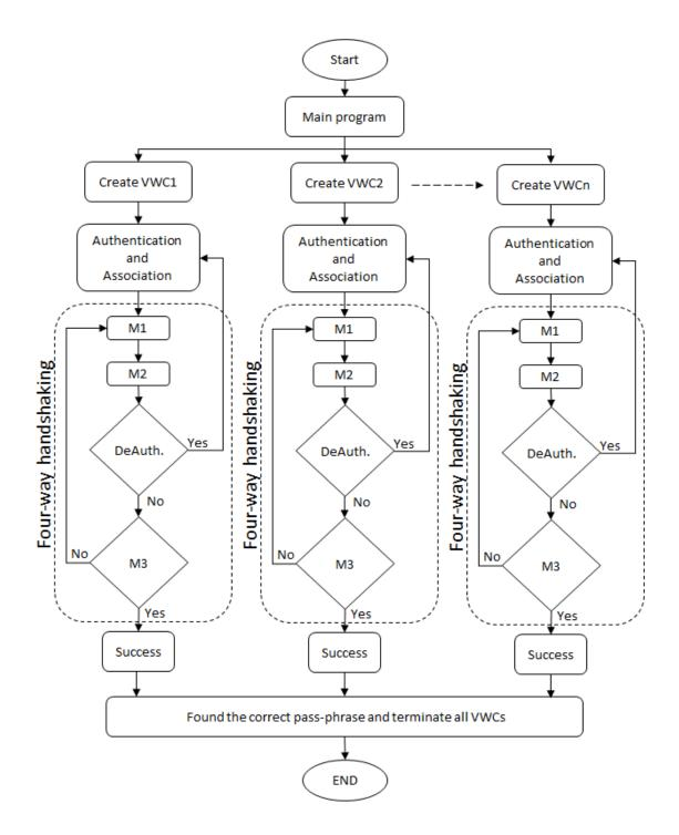
Figure 5.4: Our proposed parallel active WPA2-PSK attack design. Where M1, M2 and M3 are the first three messages of the four-way handshaking. M4 message was omitted since it is only a confirmation frame from a VWC to the AP to indicate a successful end of the four-way handshaking procedure.
