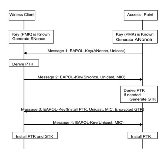
Figure 5.3: WPA2-PSK Four-Way Handshaking.
