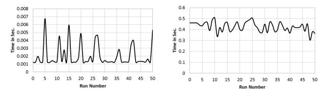
Average time for VWC1 and Figure 3.15: Average time for VWC1 and Figure 3.14: VWC2 to associate phase to RAP. VWC2 to receive DHCP configuration.
