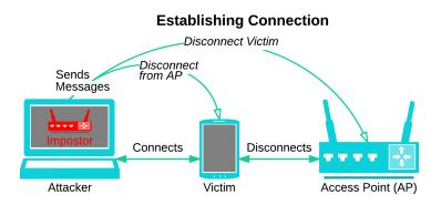
Figure 4.4: A diagram displaying how the attacker establishes connection with the victim.
