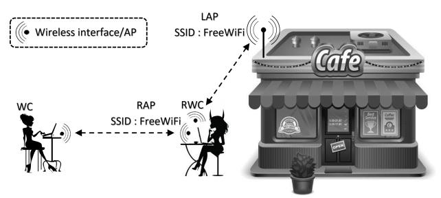
(a) Evil twin attack using single ISP gateway. The attacker pass through WC data to the Internet using LAP.
