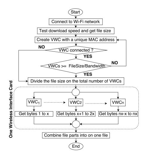
Figure 6.1: Proposed attack design on Wi-Fi hotspot traffic shaping using Virtual Wireless Clients.
