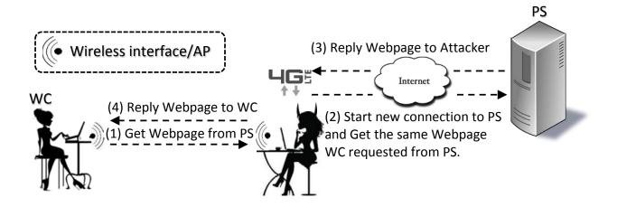
Figure 3.1: Possible man-in-the-middle attack on the ETA detection that relies on TCP connection without security.
