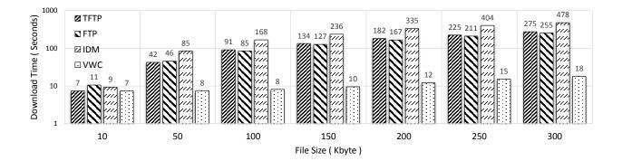
Figure 6.3: The time needed to download different files from the file server using the software in Table 6.1. Y-axis is log-10 scale.
