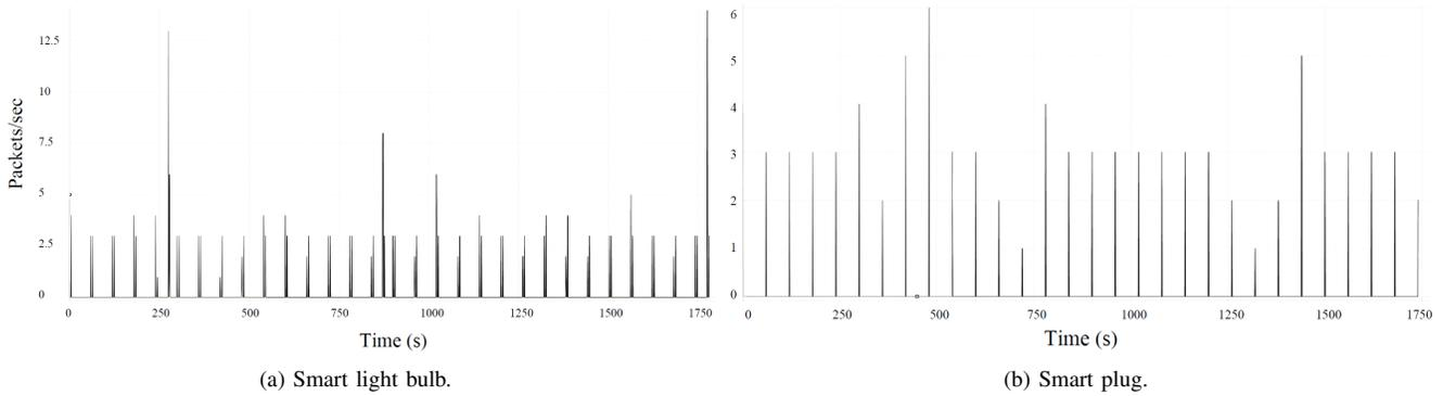
Fig. 3. Traffic flow of two devices over 30 minutes.
