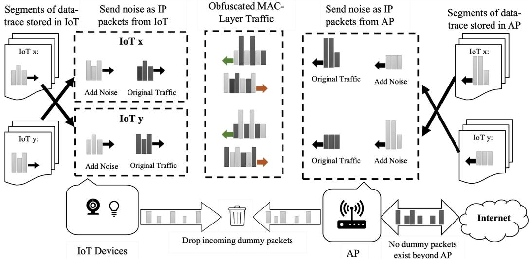
Fig. 2. WiFi traffic shaping scenario between AP and two IoT devices.
