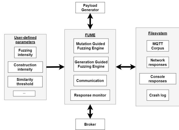
Fig. 4: FUME fuzzer architecture.
