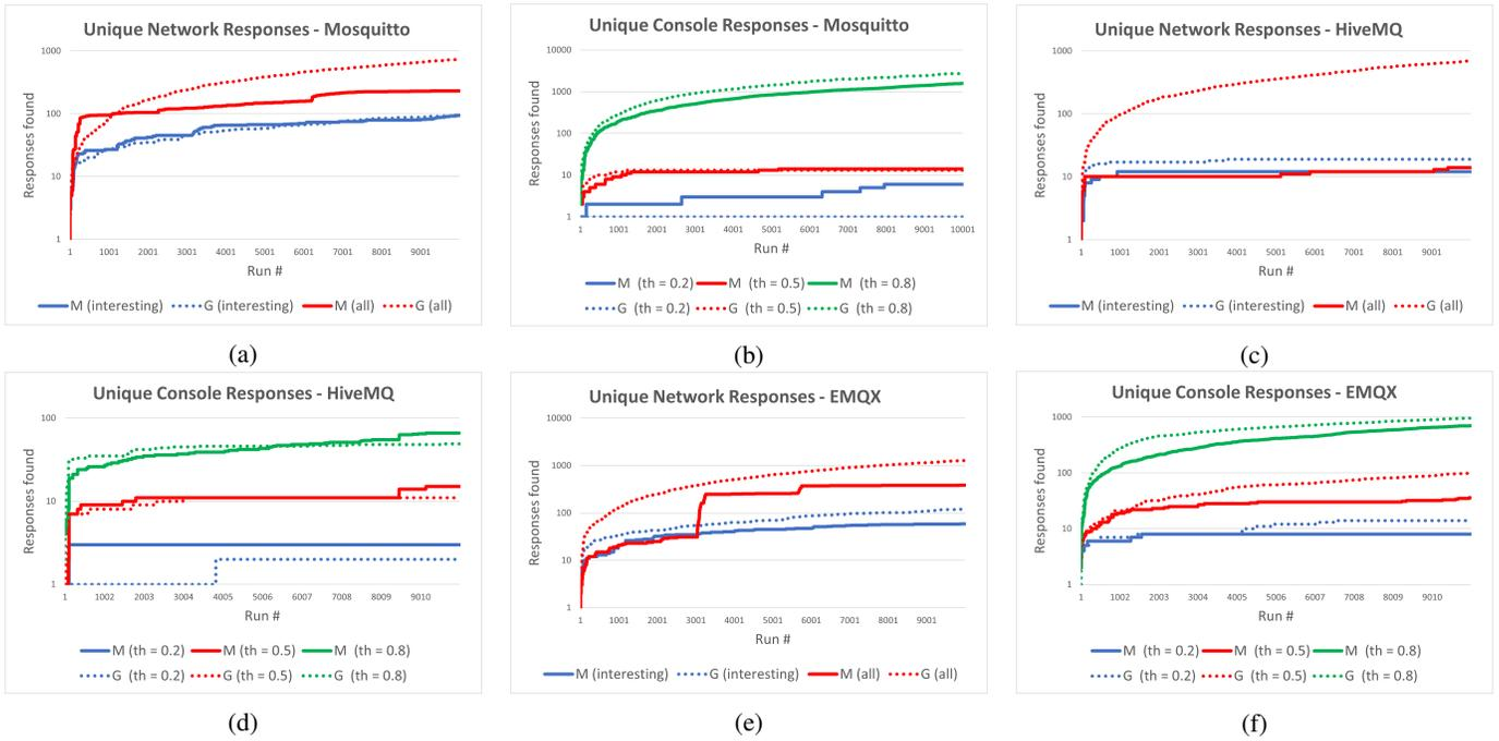
Fig. 5: State feedback evaluation – number of unique responses detected in mutation (M) versus generation (G) guided fuzzing. Tested for similarity thresholds ( $\text{th}$ ) = 0.2, 0.5, and 0.8. Interesting means that only the interesting MQTT fields were monitored, while all means that we observed all MQTT fields.
