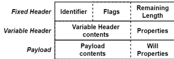
Fig. 1: MQTT packet structure. *Properties* only exists in MQTT version 5. *Will Properties* only exists in the CONNECT packet in version 5.
