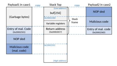
Figure 4.2: Stack-based buffer overflow attack for code injection
