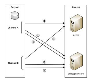
Figure 3.4: Communication Protocol between an PurpleAir Sensor and Servers.
