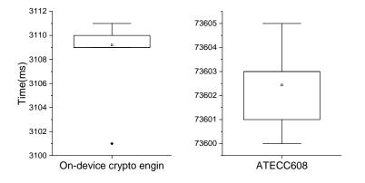
Figure 5.7: Overheads of secure boot using on-device crypto engine or ATECC608 for hashing.
