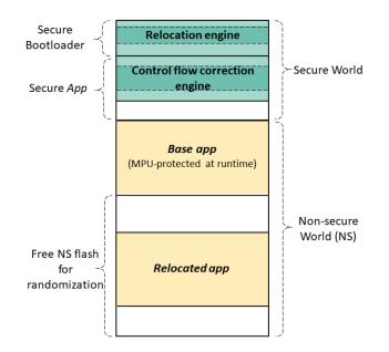
Figure 5.5: Flash layout of an iASLR-enabled system.
