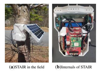
Figure 5.1: Secure and Trustworthy Air Quality Monitoring Device (STAIR).
