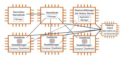
Figure 20: HDFS, YARN, and Hadoop Client Component Interfaces
