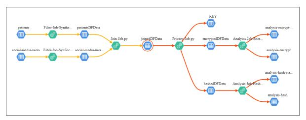
Figure 23: Data Processing and Attribute Classification Propagation in Apache Atlas
