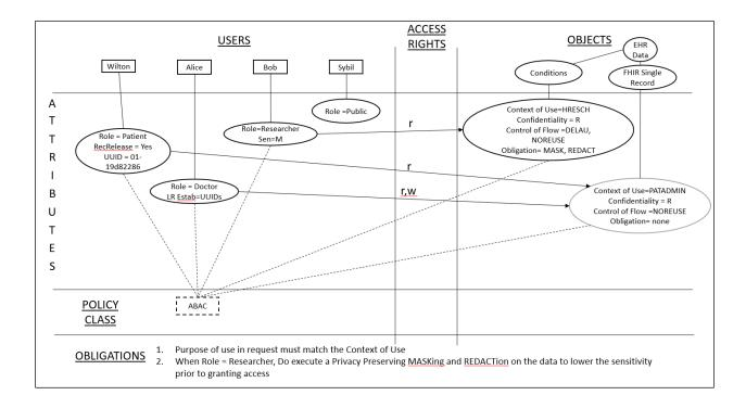
Figure 11: Example NGAC Assignment and Association Graph
