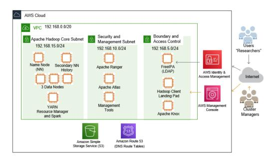
Figure 15: BDP Security Experiment Configuration
