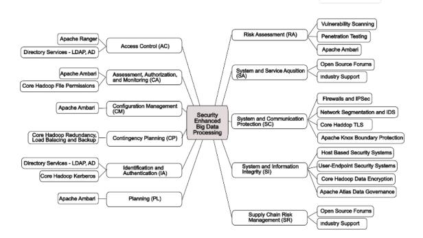
Figure 4: Mind Map: BDP Security Mechanism Mapped to RMF Security Service Controls Gateway Boundary Layer
