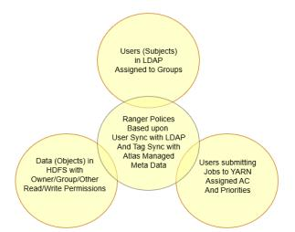
Figure 22: ABAC Implementation using HDFS, LDAP, YARN, Apache Ranger and Atlas Multiple Management Consoles
