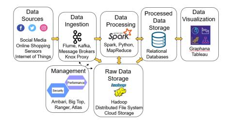
Figure 1: Overview of BDP Data Flow, Compute, and Storage Components
