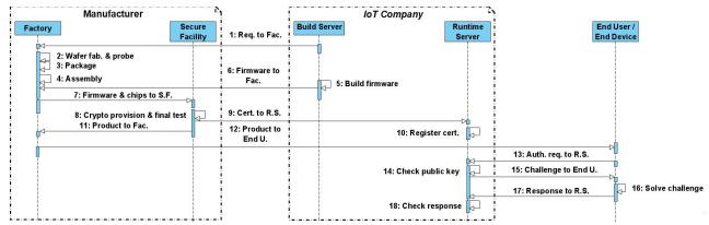
Fig. 4: Secure key provisioning framework.
