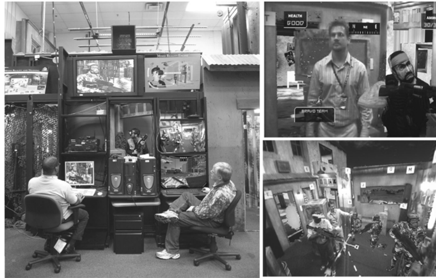
Figure 3: US Army MR MOUT facility at RDECOM, displaying multiple real, virtual or augmented views from the operator’s panel (left). Trainee observing 3D replay of the scenario with trainer (upper right). Embedded MR security camera capturing alternative views for observation (lower right) (©2006 UCF).
