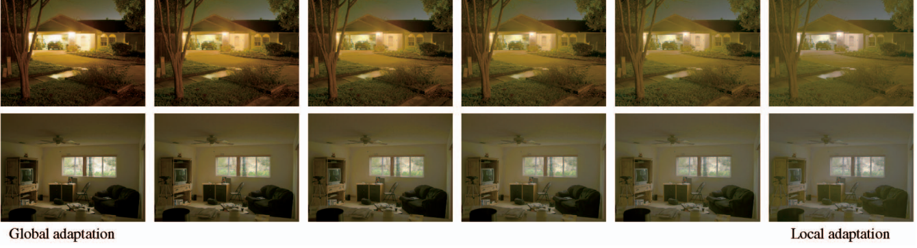
Fig. 3. Outdoor scene taken at dawn and indoor scene taken around midday, both with simulated time dependent adaptation. On the left, the adaptation level I_a is computed from the average scene luminance, whereas, on the right, the adaptation level is computed using the independent red, green, and blue components of each individual pixel.
