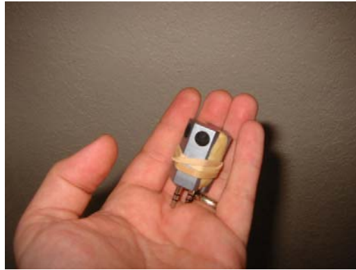
Figure 3: Miniature homemade surround microphone
