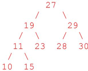
**Solution:** 6 is inserted as the left child of 10. This causes a single right rotation at node 19. During the rotation, 11 moves up to take the place of 19. Node 19 moves down, and the old right child of 11 becomes the new left child of 19.
