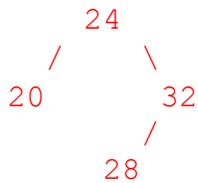
**Solution:** Inserting 29, 30, or 31 would cause a double rotation.
