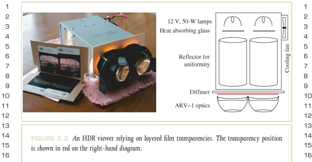
**FIGURE 5.3** An HDR viewer relying on layered film transparencies. The transparency position is shown in red on the right-hand diagram.
