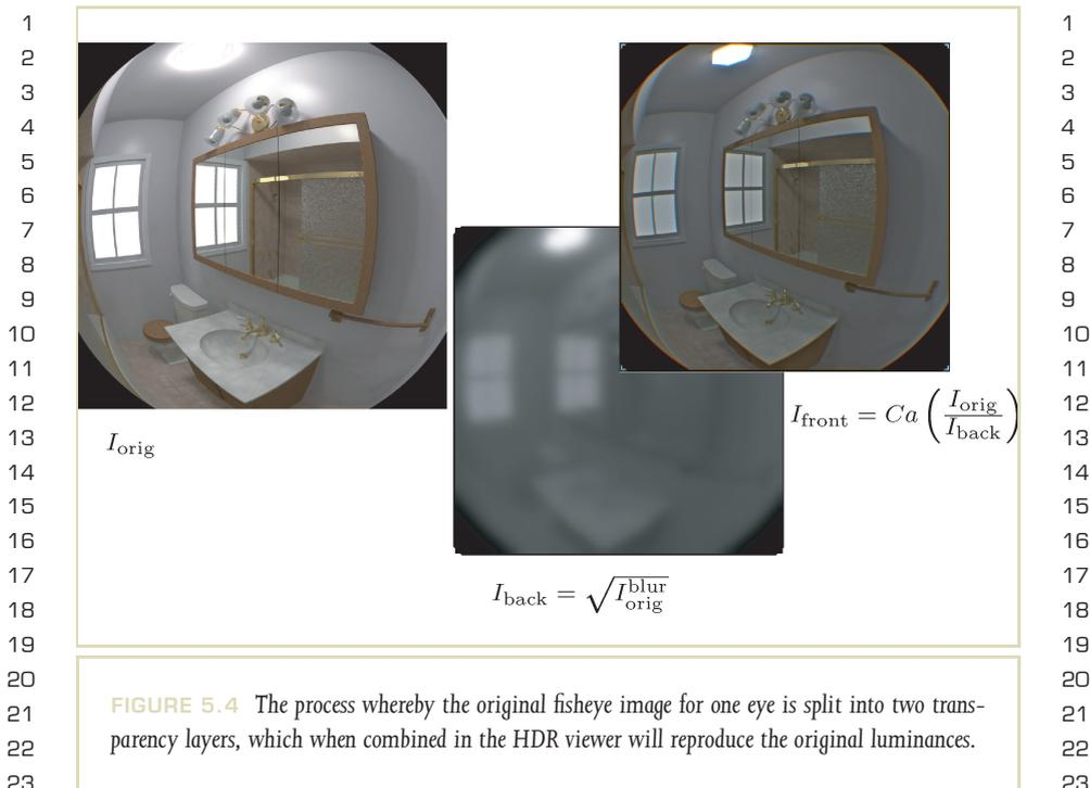
we obtain by construction the foreground image necessary to recover the original. As long as the dynamic range of the foreground transparency is not exceeded, this result is guaranteed. This method is called dual modulation.
