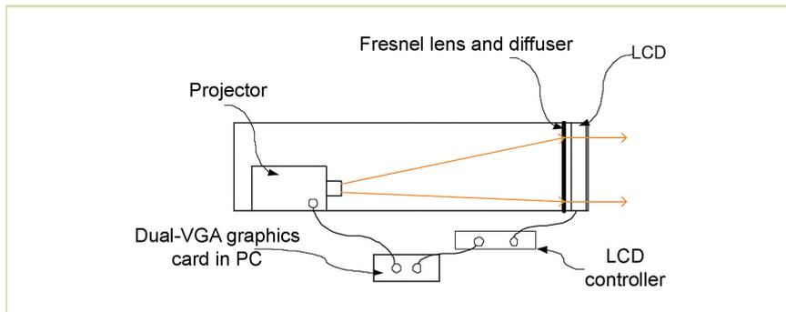
FIGURE 5.8 Sunnybrook Technologies' projector-based display [114].
