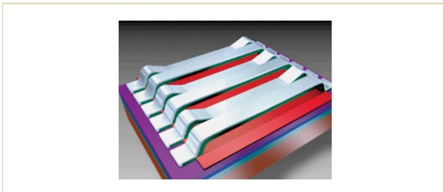
**FIGURE 5.11** Silicon Light Machines' micrograting (GLV) pixel. Each ribbon is about 5 microns wide.
