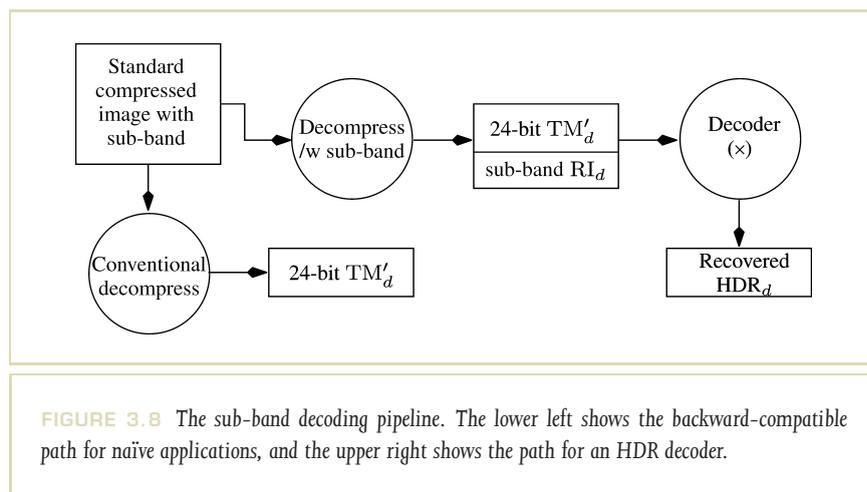
FIGURE 3.8 The sub-band decoding pipeline. The lower left shows the backward-compatible path for naïve applications, and the upper right shows the path for an HDR decoder.
