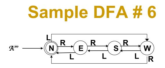
$\mathcal{A}^{""} = (\{N, E, W, S\}, \{R, L\}, \delta^{""}, N, \{N\}), where \delta^{""}$  is defined by above diagram.  $L(\mathcal{A}^{""}) = \{w \mid w \text{ is a set of commands passed to a sentinel that starts facing North and changes directions R(ight)/clockwise or L(eft)/counterclockwise based on the corresponding input character. w must eventually lead the sentinel back to facing North }$
