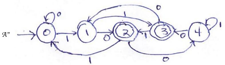
$\mathcal{A}^{"} = (\{0,1,2,3,4\}, \{0,1\}, \delta^{"}, 0, \{2,3\}), \text{ where } \delta^{"} \text{ is defined by above diagram. } L(\mathcal{A}^{"}) = \{ w \mid w \text{ is a binary string that, read left to right (msb to lsb), when interpreted as a decimal number divided by 5, has a remainder of 2 or 3 }$
