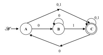
Using the technique of ripping (collapsing) states, replacing transition letters by regular expressions, develop the regular expression associated with  $\mathcal{L}$  that generates L. I have included the diagrams associated with removing states A, B, then C, in that order.
