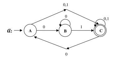
Using the technique of ripping (collapsing) states, replacing transition letters by regular expressions, develop the regular expression associated with a that generates L. I have included the diagrams associated with removing states A, B, then C, in that order.
