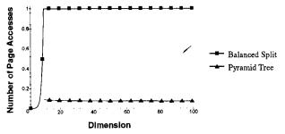
Figure 12: Number of page accesses when processing range queries for the Pyramid Tree and Balanced Splitting
