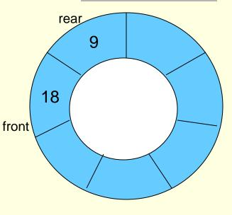
visualization of a queue implemented as a circular array after dequeue operation
