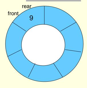
visualization of a queue implemented as a circular array after dequeue operation
