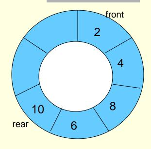
visualization of a queue implemented as a circular array after insertion of element 10
