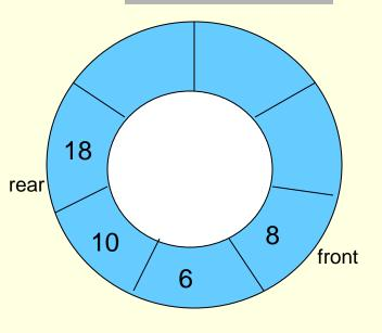
visualization of a queue implemented as a circular array after dequeue operation
