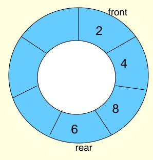
visualization of a queue implemented as a circular array after insertion of element 6
