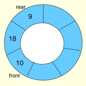
visualization of a queue implemented as a circular array after insertion of element 9
