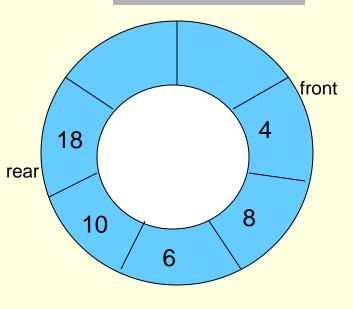
visualization of a queue implemented as a circular array after insertion of element 18
