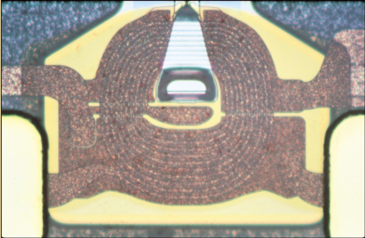
Optical micrograph of an IBM giant magnetoresistive head for writing and reading data on a computer's magnetic hard disk drive
