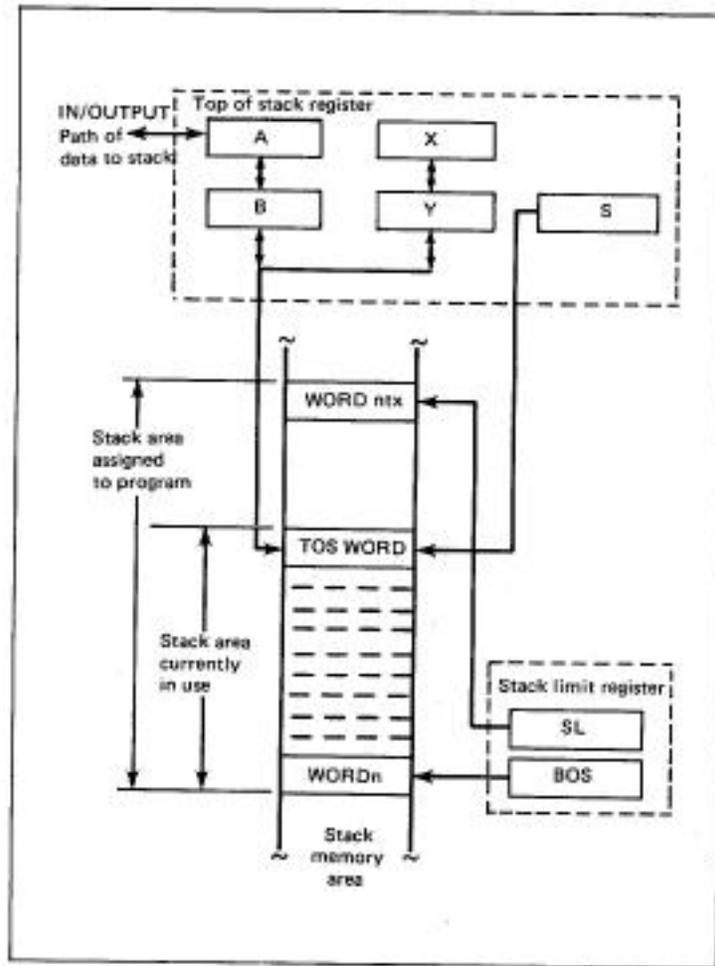
Fig. 2. Top of stack and stack bounds registers.
