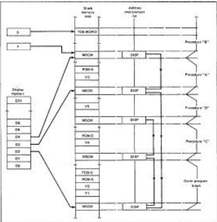
Fig. 5. Display registers indicating current addressing environment.
