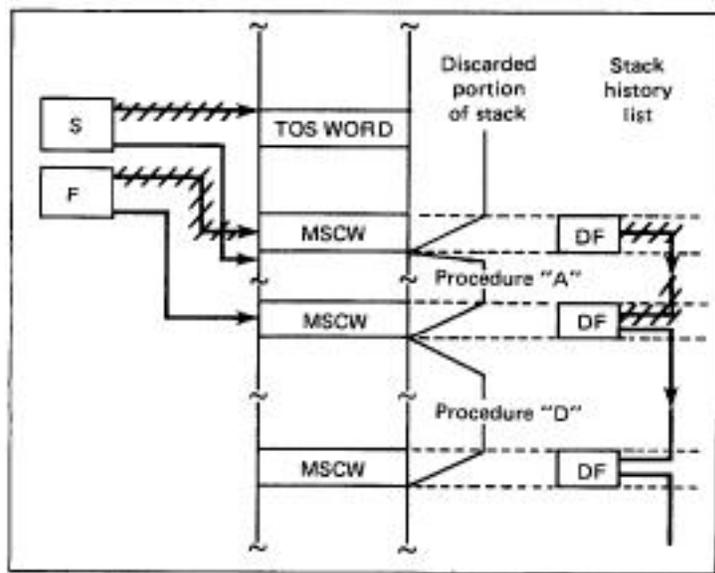
Fig. 4. Stack cut-back operation on procedure exit.
