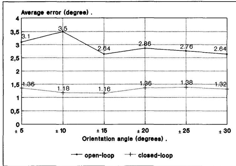
Fig. 3. Average errors of the closed-/open-loop algorithm for baseline detection and correction.
