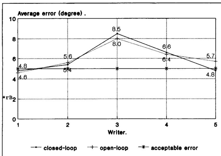
Fig. 6. Average error of the slant estimation algorithm: open loop vs. closed loop.
