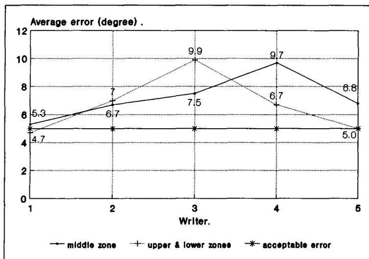
Fig. 5. Average error of the slant estimation algorithm: comparison between zones.
