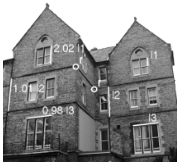
Fig. 8. Measuring ratio of lengths of parallel line segments lying on two parallel scene planes: The points r and r' (together with the plane vanishing line and the vanishing point) define the homology between the two planes on the facade of the building.
