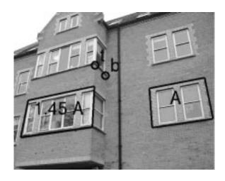
**Figure 7: Measuring ratios of areas on separate planes:** The image points **t** and **b** together with the vanishing line of the two parallel planes and the vanishing point for the orthogonal direction define the homology between the planes. The ratio between the area of the window on the left plane and that of the window on the right plane is computed.
