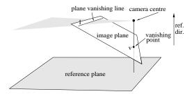
**Figure 1: Basic geometry:** The plane's vanishing line l is the intersection of the image plane with a plane parallel to the reference plane and passing through the camera centre. The vanishing point v is the intersection of the image plane with a line parallel to the reference direction through the camera centre.
