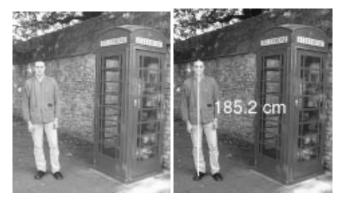
**Figure 10:** Measuring the height of a person in an outdoor scene: The ground plane is the reference plane, and its vanishing line is computed from the slabs on the floor. The vertical vanishing point is computed from the edges of the phone box, whose height is known and used as reference. The veridical height is 187cm, but note that the person is leaning slightly on his right foot.
