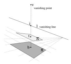
**Figure 2:** Cross ratio: The point **b** on the plane  $\pi$  corresponds to the point **t** on the plane  $\pi'$ . They are aligned with the vanishing point **v**. The four points **v**, **t**, **b** and the intersection **i** of the line joining them with the vanishing line define a cross-ratio. The value of the cross-ratio determines a ratio of distances between planes in the world, see text.
