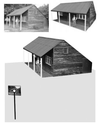
**Figure 12:** Complete 3D reconstruction of a real scene: (left) original image; (right) a view of the reconstructed 3D model; (bottom) A view of the reconstructed 3D model which shows the position of the camera centre (plane location X,Y and height) with respect to the scene.
