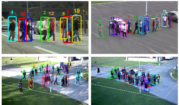
Figure 1. Tracking results using the proposed joint detector on four public datasets: (clockwise) TUD-Crossing, ParkingLot, PETS S2.L2 and PETS S1.L2.
