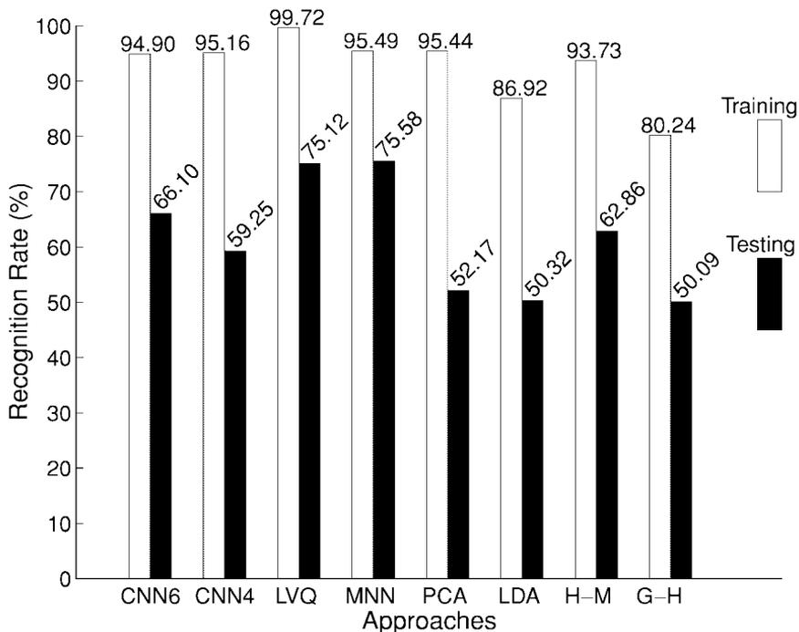
**FIG. 8.** Typical results obtained using different techniques. The gray bars are for the training set, and the black ones for the test set. CNN4 and CNN6 stand for four- and six-layered CNNs, respectively. H-M and G-H stand for Hausdorff metric-based and geometric hashing-based approaches, respectively.
