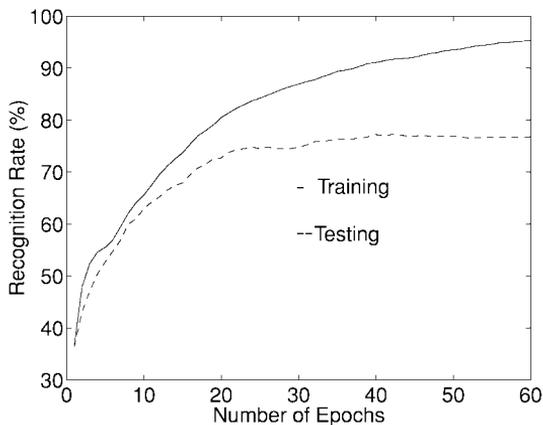
**FIG. 9.** The learning curves of a CNN, when trained with the test set, and tested with the training set (only with those five target types available in the test set).
