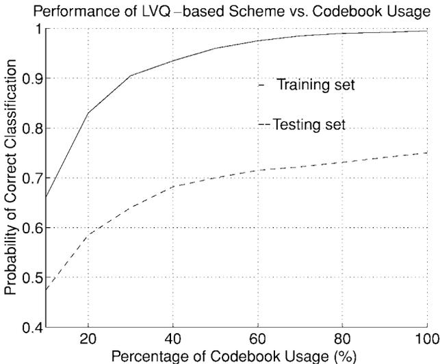
FIG. 6. The performance curve of the LVQ-based classifier as shown in Fig. 5.
