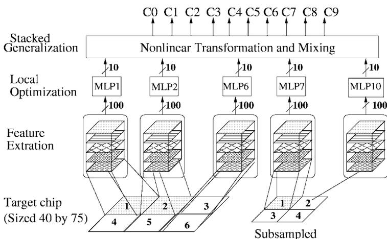
**FIG. 7.** The Modular Neural Network-based scheme evaluated in this paper.
