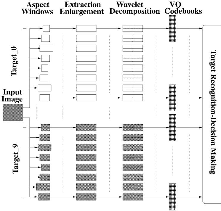
FIG. 5. The Learning Vector Quantization-based scheme evaluated in this paper.
