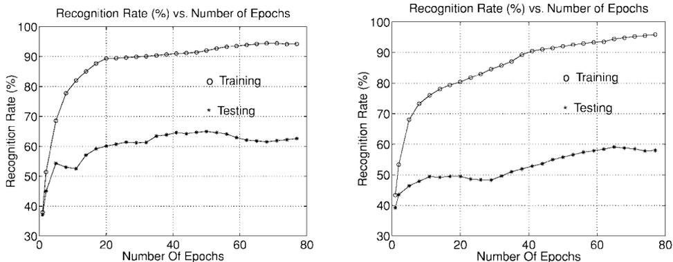
**FIG. 4.** Learning curves and recognition rates for a six-layered CNN (left) and a four-layered CNN (right), respectively (plotted every three epochs).
