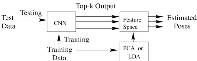
**FIG. 11.** A hierarchical pose estimator.
