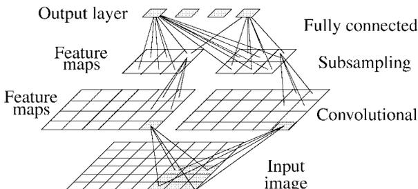
FIG. 1. A typical configuration for convolutional neural networks.
