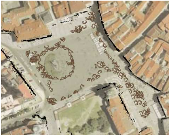
Figure 4: Example registration of cameras to an overhead map. Here, the cameras and recovered line segments from the Prague data set are shown superimposed on an aerial image. (Aerial image shown here and in Figure 5 courtesy of Gefos, a.s. ( www.gefos.cz ) and Atlas.cz.)
