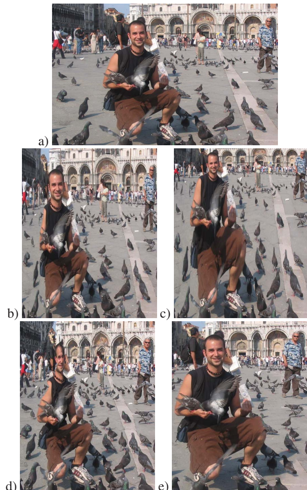
Figure 1. Comparison of a few retargeting methods, reducing width by half. (a) Original image. (b) Video-retargeting [19]; (c) Optimized scale-and-stretch [16]; (d) Improved Seam Carving [13]; (e) Our shift-map editing.
