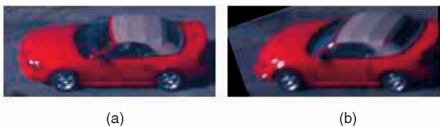
Fig. 18. Quasi-rigid alignment results for the pair of images in Fig. 10 ((a) original model image, (b) warped query image). The pose change is around 33^\circ .
