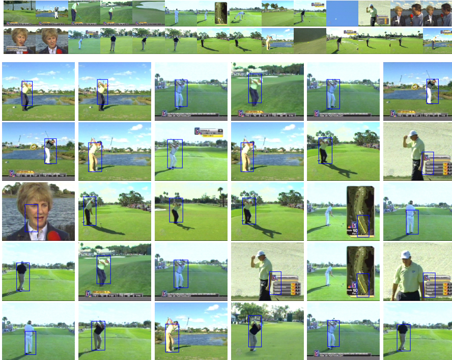
Fig. 8. The top 30 detections for a 8-frame swing template action in an 8000-frame video golf . There are 10 hits (with duplicates) of 14 true positives and 11 false positives, yielding 71% recall and 63% precision. This is a difficult video with few true positives compared to negatives, and much camera motion.
