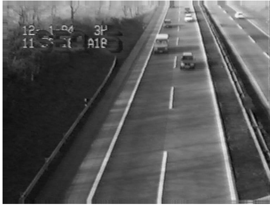
Fig. 1. A traffic surveillance example. This is a typical camera image from a traffic surveillance camera. Notice that especially for dark coloured cars intensity differences between foreground and background are small. In order to track the cars robustly it is necessary to detect the shadows as well as the cars.
