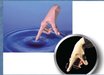
A tactile device that puts vibrating actuators on the fingertips and the palm of the hand. (Photograph reproduced by permission of Immersion Corporation, © 2004 Immersion Corporation. All rights reserved)
