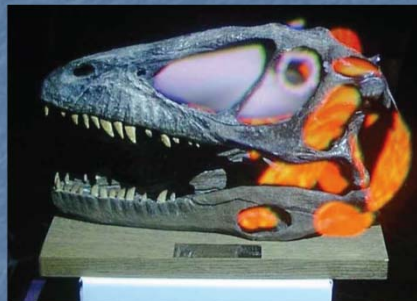
The Virtual Showcase, an augmented surface display that projects virtual information onto a physical 3D artifact, presenting a seamless integration of the physical object and virtual content. (Photograph courtesy of Oliver Bimber)
