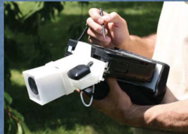
HYDROSYS handheld AR device setup. (Image courtesy of Ernst Kruijff and Eduardo Veas)
