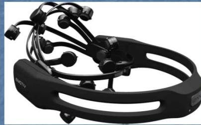
Head-worn 14 channel brain-computer input device that reads EEG information from strategically placed points on the scalp (Photograph courtesy of Emotiv)
