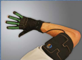
A bend-sensing data glove that can track the fingers. (CyberGlove Model III photograph courtesy of CyberGlove Systems)
