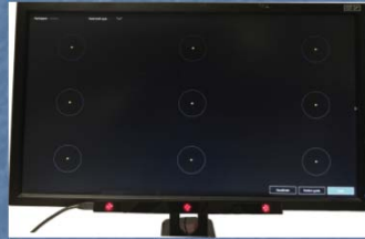
Passive eye-tracking device that does not require the user to wear anything (Photograph courtesy of Joseph J. LaViola Jr.)
