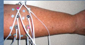
An example of EMG sensors applied to a user's forearm. (Photograph courtesy of Desney Tan, Microsoft Research)
