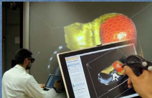
The Eye of Ra hybrid interface, combining 2D and 3D interaction. (Image courtesy of Ernst Kruijff)
