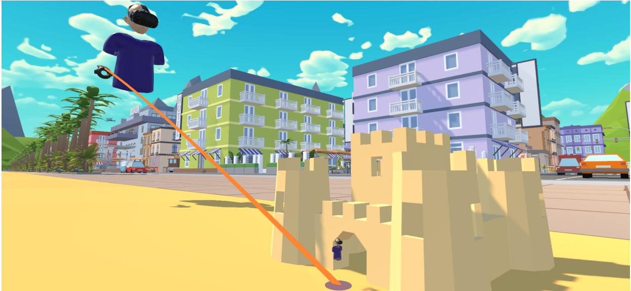
Fig. 1: We present three novel teleportation-based travel techniques that enable users to adjust their scale in the virtual environment, thereby affecting their modeled eye distance and height. In our Simultaneous technique shown in this picture, the user adjusts the scale of a preview avatar while selecting its new horizontal position with a parabolic selection ray known from same-scale teleportation techniques. Upon confirmation, the user is instantaneously teleported to the indicated position and scale.
