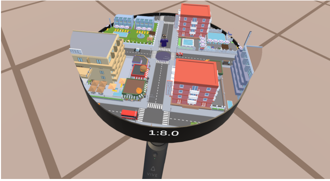
Fig. 2: When planning a teleport with scale changes, the new surroundings of the user are previewed by a circular cutout from a World-in-Miniature (WIM) attached to the user’s controller in the non-dominant hand. The preview avatar has a fixed size, and the size of the surrounding objects adjusts based on the currently selected scale.
