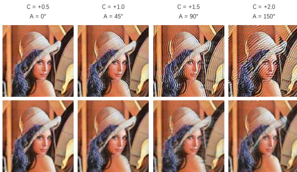
Figure 5: Pre-correction with different hyperopia parameter C and A . The top row shows the pre-corrected images and the bottom row shows the simulated retinal images.
