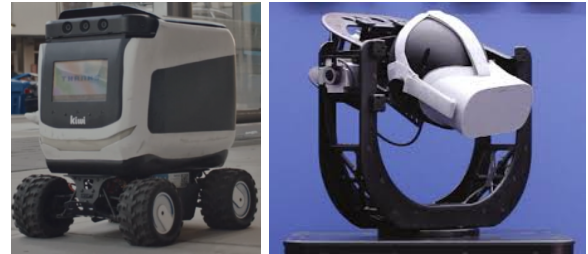
Fig. 1: (a) A Kiwibot food delivery robot. (b) A robot in full VR: An Optofidelity Buddy 3 wearing an Oculus Go headset.
