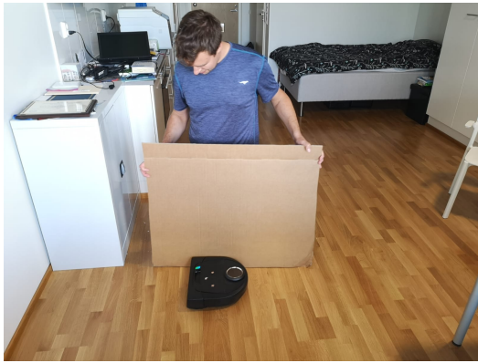
Fig. 4: A human (Markku) with cardboard, acting as a VWG, haptic renderer and display for a Neato vacuum cleaner robot.
