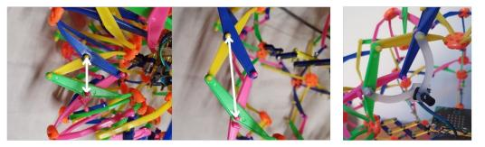
**Figure 3.** (Left) Change in angle of SLE when open versus closed; (**Right**) potentiometer mounted as an auxiliary SLE.
