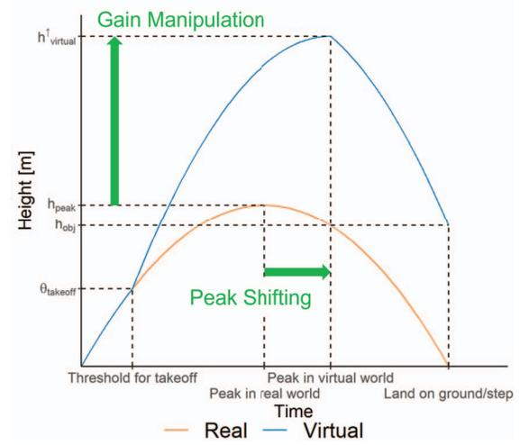
Figure 3: Theoretical position changes with gain manipulation and peak shifting applied.
