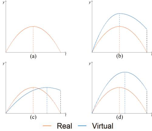
Figure 2: Changes in the user’s height with (a) no manipulation, (b) gain manipulation, (c) peak shifting, and (d) both. The peak height in reality and the landing height in VR are the same for all four figures.
