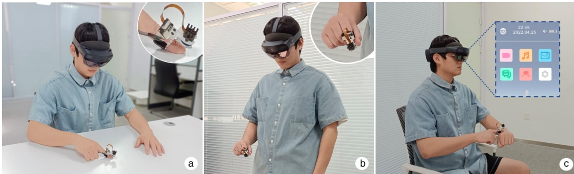
Figure 1: NailRing is an intelligent finger ring that recognizes micro gestures based on fingertip physiological characteristics to achieve interactive input in MR. (a) The user wears the NailRing on a flat surface to perform interaction tasks by fingertip micro-gestures; (b) In the walking state, the user responds quickly to interaction requirements by one-handed gestures; (c) The user interacts with the MR application through the NailRing with the back of the auxiliary hand as the interaction plane.
