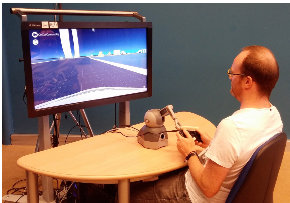
Figure 3: Proof-of-concept setup, based on a large screen and a gamepad attached to a 3DOF haptic device.
