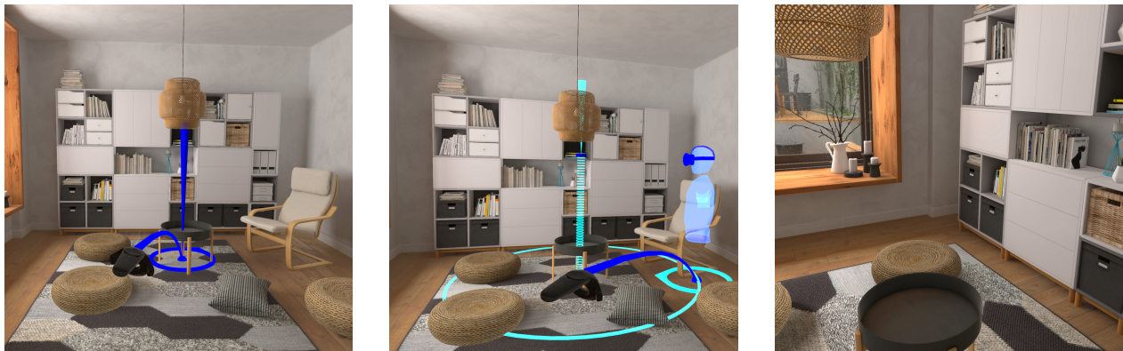
Figure 1: Anchored Jumping allows a user to specify a rotation axis (left) and a new viewing position relative to it (middle). The user will then teleport to the indicated viewing position and automatically face the specified rotation axis (right). Depending on the scenario, this axis can either be re-activated for the next maneuvering step or be re-specified for each jump.
