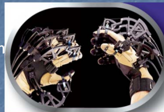
A body-referenced force-feedback device. (Photograph reproduced by permission of Immersion Corporation, © 2004 Immersion Corporation. All rights reserved)
