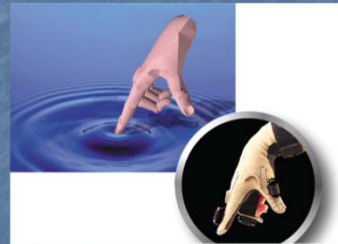
A tactile device that puts vibrating actuators on the fingertips and the palm of the hand. (Photograph reproduced by permission of Immersion Corporation, © 2004 Immersion Corporation. All rights reserved)
