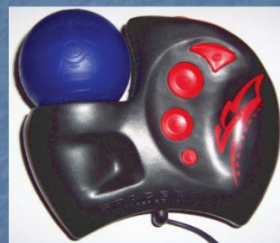
An isometric 3D input device. (Photograph courtesy of Andrew Forsberg, Brown University Graphics Group)
