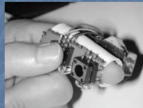
A user pressing one of the multilevel buttons on the FingerSleeve. (Photograph reprinted from Zeleznik et al. (2002), © 2002 IEEE Press)
