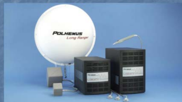
Magnetic sensor consists of an electronics unit, a magnetic field generator, and receivers that track the user or object. (Photograph courtesy of Polhemus Inc.)
