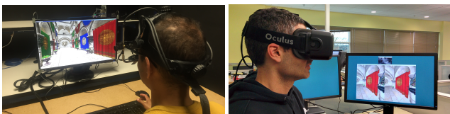
Figure 7: Our user study Setups. Left shows our desktop setup with a high-speed gaze tracker, and right is our HMD setup with a gaze-tracker integrated within the HMD.
