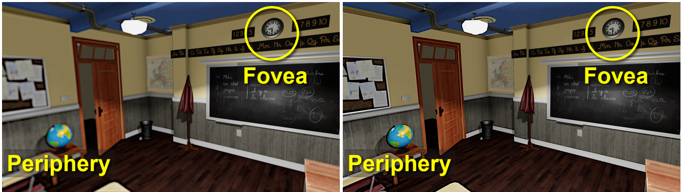
Figure 1: Our classroom scene with eye fixation at the yellow reticle. (Left) Our perceptually-validated target foveated image. (Right) Our proposed foveated rendering system that avoids shading up to 70% of the pixels and closely matches the frequency content of our target by using pre-filtered shading terms, contrast preservation, and applying a new temporal antialiasing that improves temporal stability by an order of magnitude (providing stability similar to a temporally antialiased non-foveated renderer). The original version of the classroom scene is courtesy of Christophe Seux.
