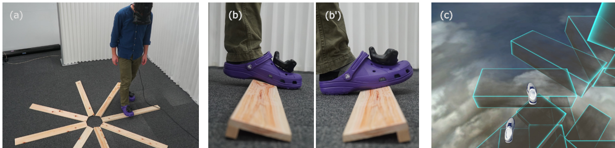
Fig. 1: Overview of the proposed system that enabled the user to ascend and descend spiral stairs infinitely in the virtual environments (VEs). (a) The user steps on small bumps attached to a flat floor in the real space corresponding to the edge of steps in the VEs. The user feels a strong sensation of ascending and descending by stepping on the small right-angled bumps (i.e., ascending case: (b), descending case: (b')). (c) The visual stimuli that simulated staircase walking provides via head-mounted displays.
