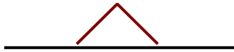
Fig. 6: Schematic of the bumps set on the floor with the corner turned up.
