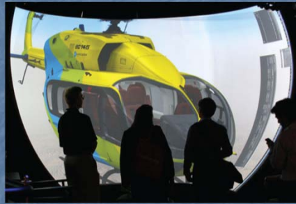
A curved, rear-projected surround-screen display that combines both hemispherical and cylindrical geometry. (Photograph courtesy of Digital Projection)
